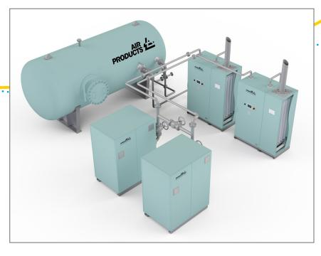
The NC 1.3 Nitrogen Generator is a PRISM® membranebased nitrogen generator which is designed specifically for shipboard use. This robust cabinet system has the capacity to supply up to 420 cubic meters of nitrogen per hour, is DNV Type-A approved, and meets demanding international marine standards.
