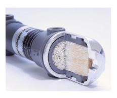
Each membrane separator contains thousand of tiny hollow fiber membranes which use selective permeation to separate nitrogen and oxygen molecules and route them into individual streams.
